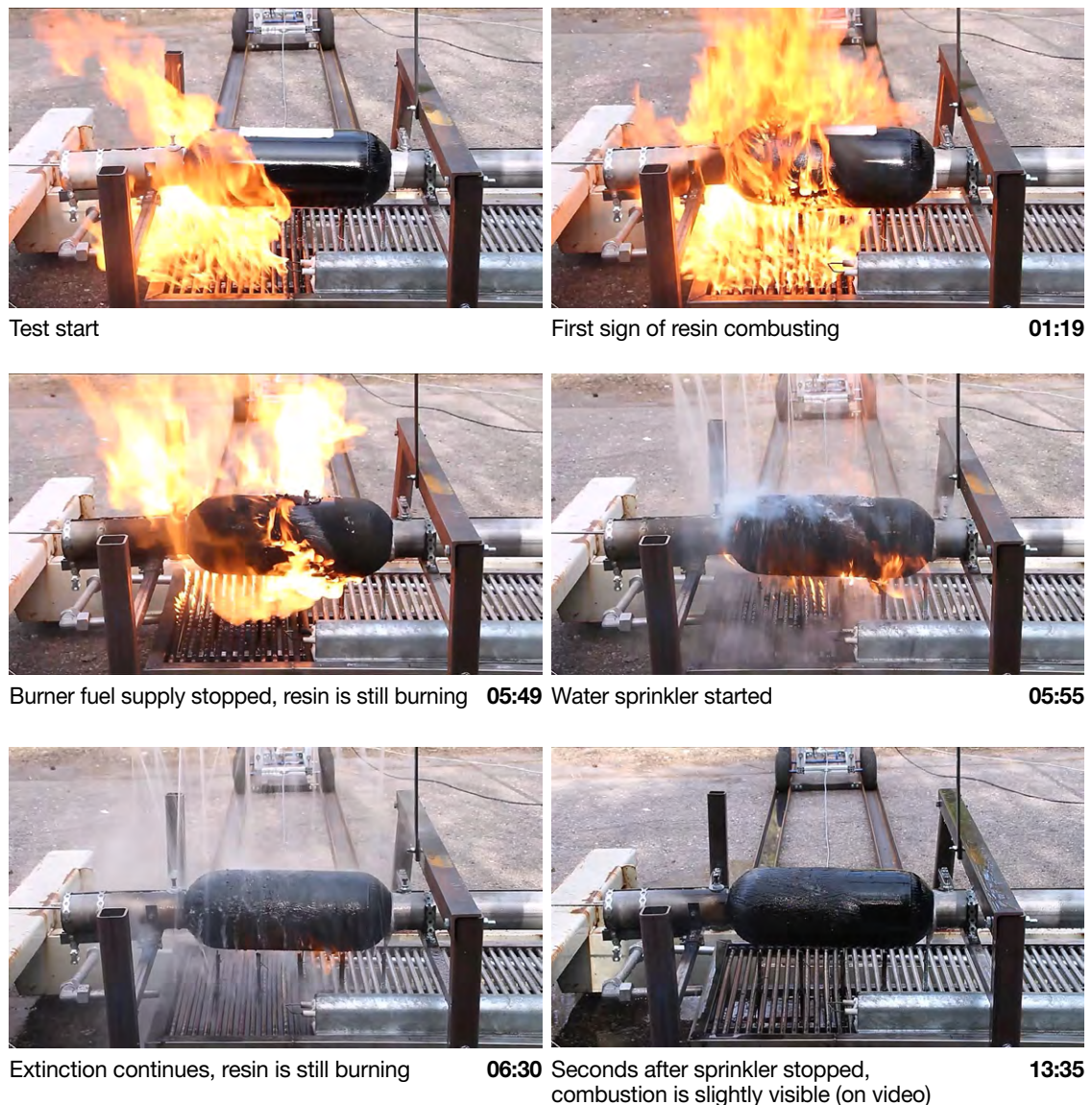
Figure 2. Self-venting tank prototype in a fire with flame extinction 29 .
