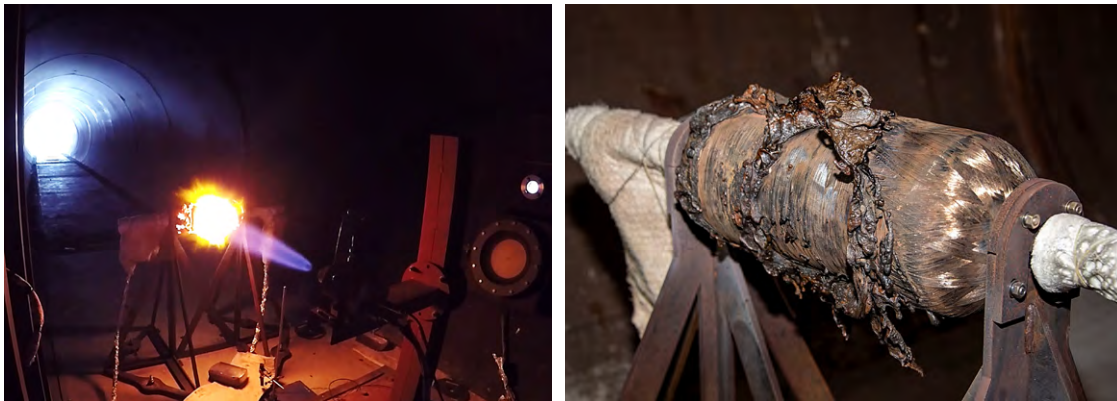
Figure 3. Self-venting tank prototype under extreme impinging jet fire of highest ever intensity of HRR/A=19.5 \text{ MW/m}^2 from a 700-bar storage tank: left – during fire test, right – aftermath of the prototype composite of tank test 30 .
